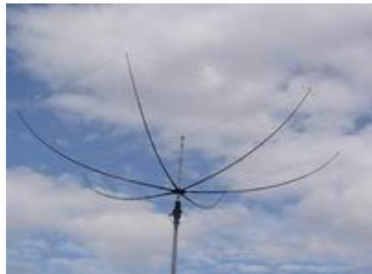
A consequence of bending the driven element and reflector into the W shape is to increase their Q. I measure a value of about 30 for a 10m Hexbeam reflector, compared to 10 for the equivalent linear element. The result is a relatively narrow performance bandwidth.
